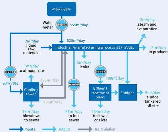
Water inputs and outputs for an example industrial site
