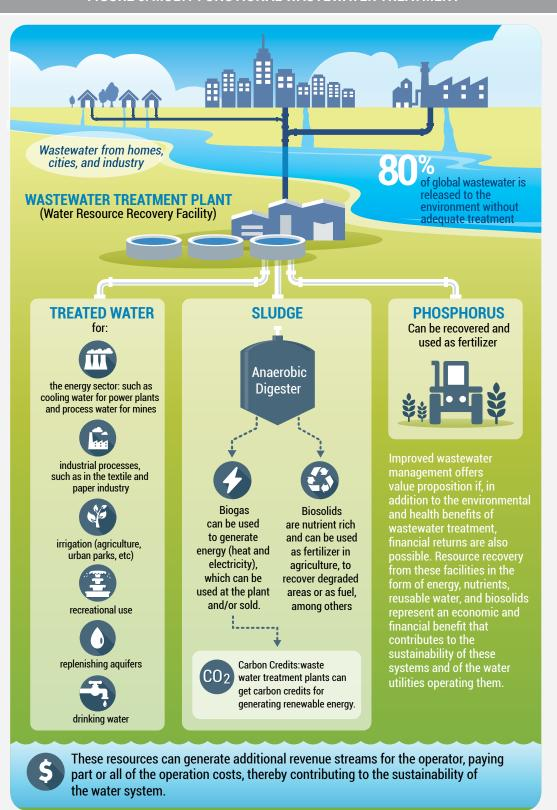
FIGURE 6: MULTI-FUNCTIONAL WASTEWATER TREATMENT
